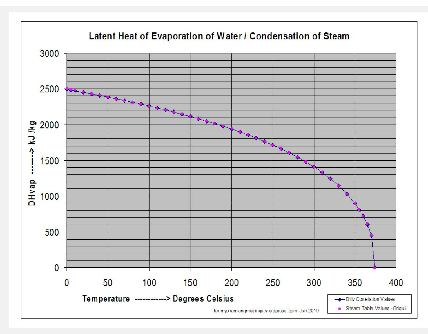
Latent Heat of Evaporation/Condensation of Water as function of temperature
